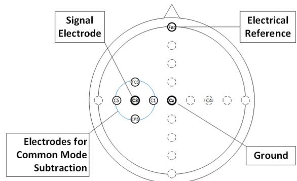
Fig. 2. **EEG Electrode Positions:** Map of EEG electrodes used. Ground was placed at Cz in the middle of the head. Electrical reference is on the forehead at Fpz. Sensing of motor intention was done with an electrode placed at C3 with a ring of electrodes surrounding it for common-mode subtraction.
