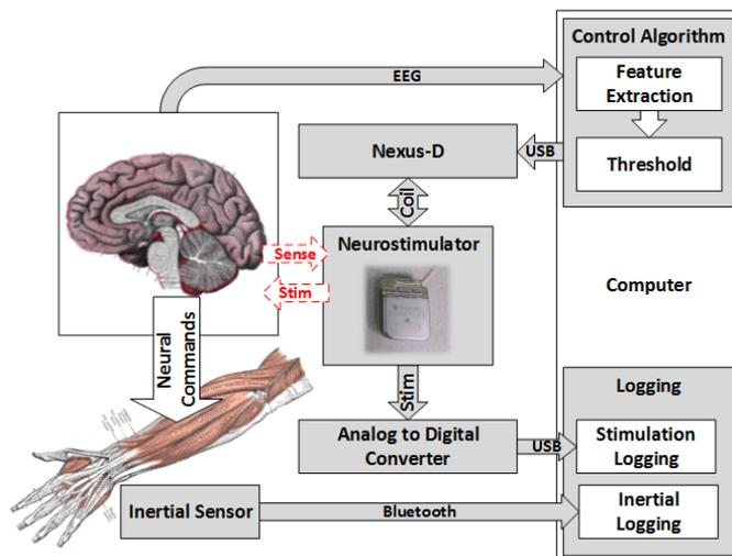
Fig. 1. **Experimental Setup:** A system block diagram showing the connections between various components for this experiment. Grayed blocks are used in this proof-of-concept setup. Dashed lines indicate the ability for a future implanted system to perform sensing and stimulation directly without need of worn EEG.
